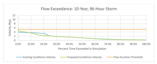
Figure 7 Velocity exceedance plot for the 10-Year, 96-Hour storm
