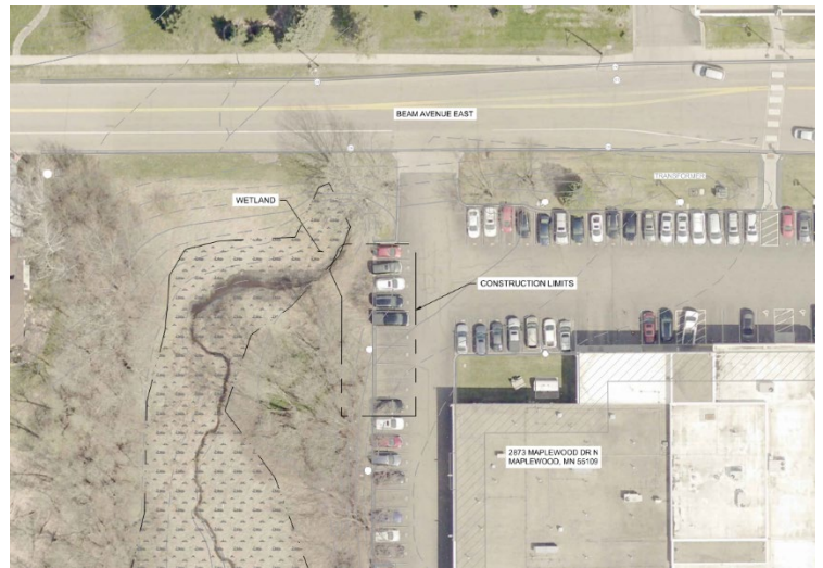
Figure 1: Maplewood Toyota's BMP is a pretreatment structure to reduce pollutants being deposited directly into the wetland that flows into Kohlmann Lake.
