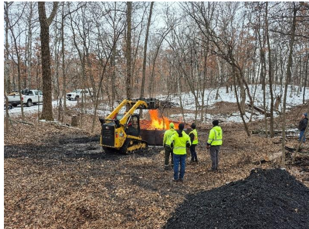
A skid steer operator places woody biomass into a biochar kiln as staff look on. The biochar end product is in the foreground.
