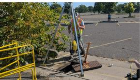
On September 13, 2024, RWMWD staff conducted a "synthetic storm" test on two of the trenches in the south tree grove. The purpose of this test was to evaluate the capacity of tree trenches to reduce stormwater volume during a storm event. Two of the tree trenches in the south grove were flooded with 15,575 gallons of using water from a fire hydrant on site. Outflows were monitored over the next 6 hours with monitoring equipment.
