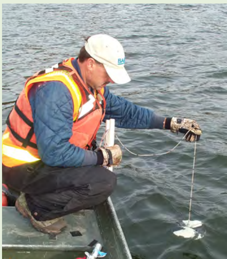
Measuring water clarity with a Secchi disc
