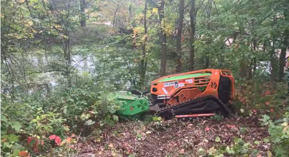
A remote-control brush mower was tested on a steep slope. The results were encouraging.
