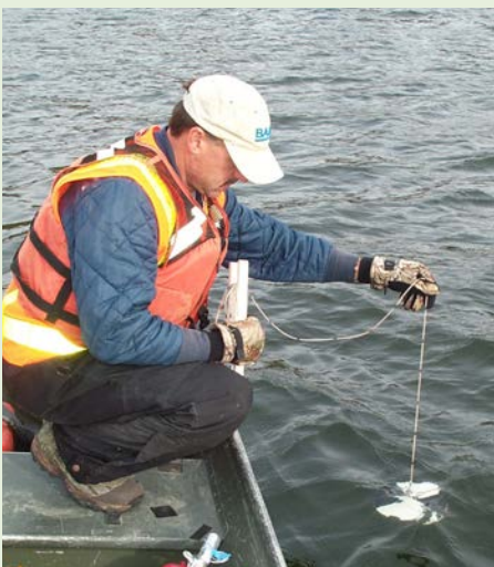
Measuring water clarity with a Secchi disc
