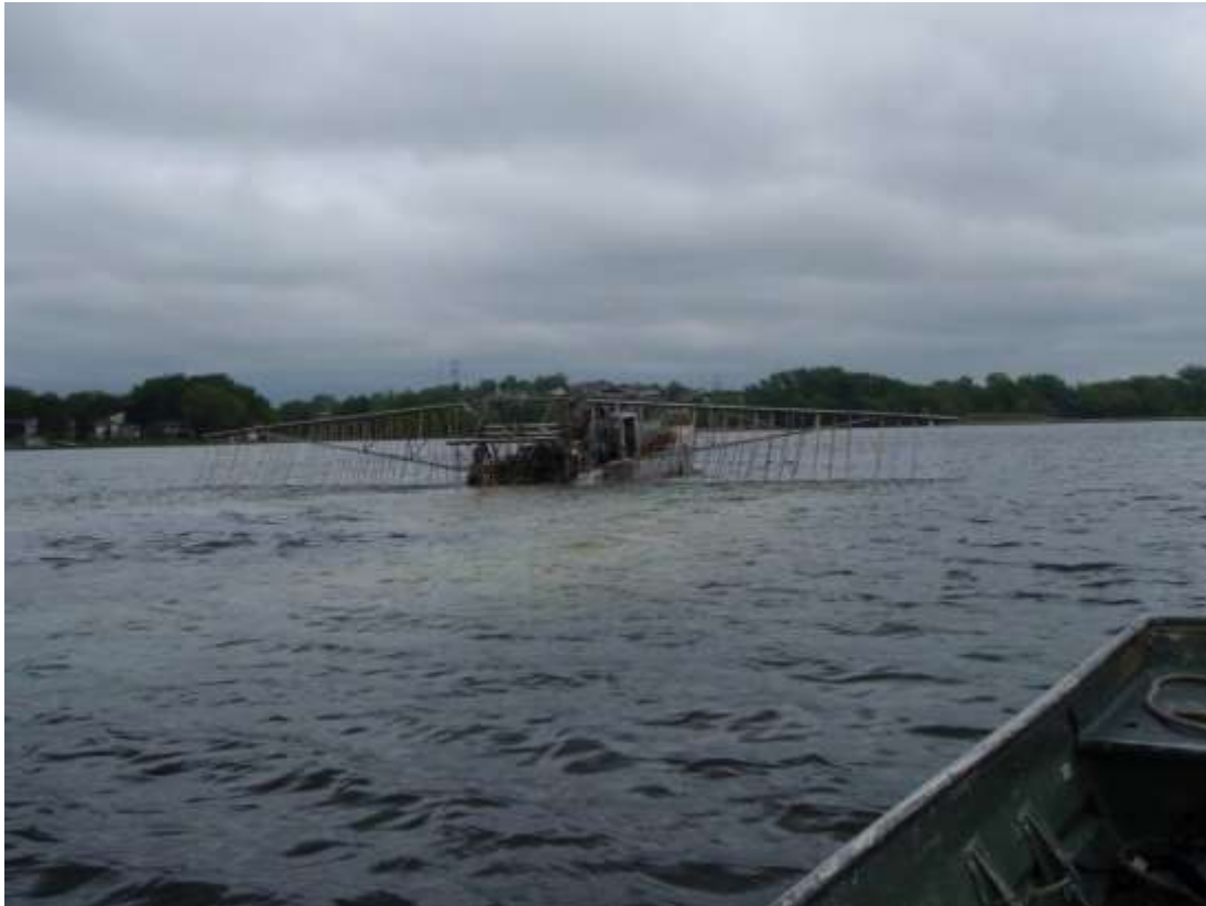
Figure 3: Alum Treatment Being Applied on Kohlman Lake (2010)
