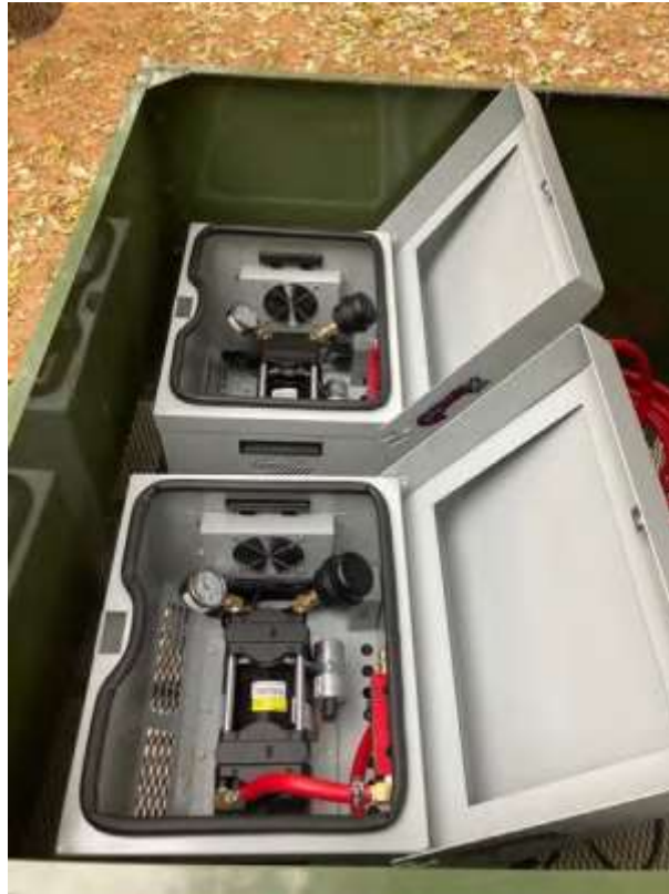
Two compressor pumps generate air flow.
