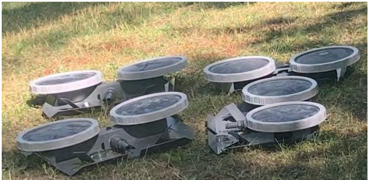
Four twin diffuser heads ready for deployment.
