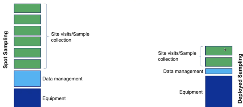
Figure 3: In-Situ qualitative cost comparison between spot sampling and deployed sampling
