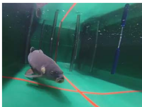
Figure 7: Common carp turning away from the NEPTUN system ( http://fishprotection.eu/ )
