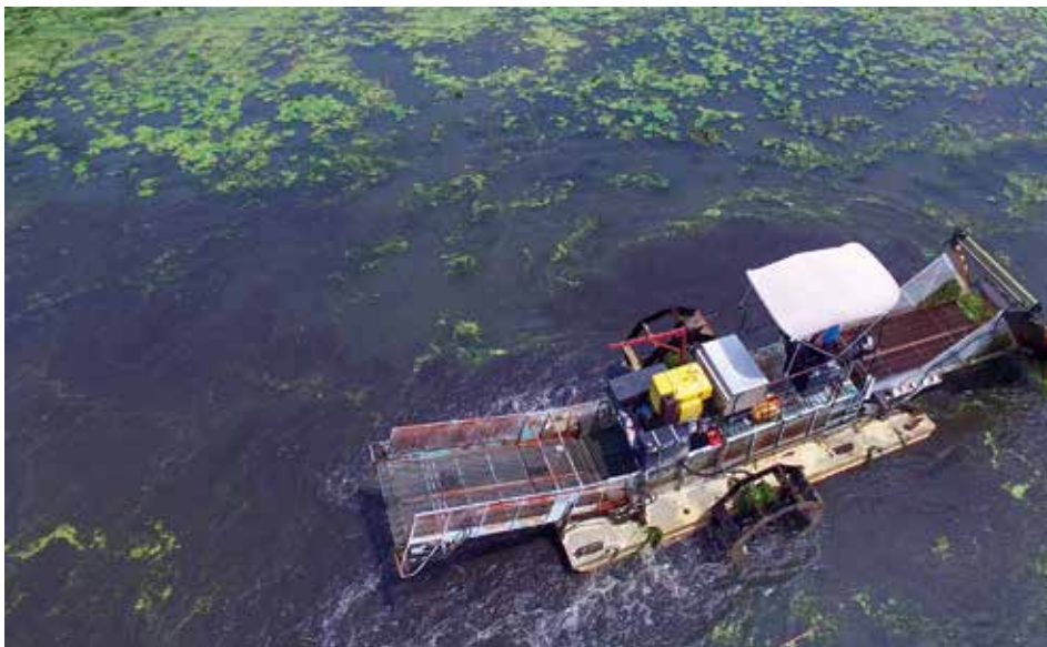
Figure 9. An aquatic plant harvester was used to cut one foot under the water and collect a mix of filamentous algae and submersed vegetation.
