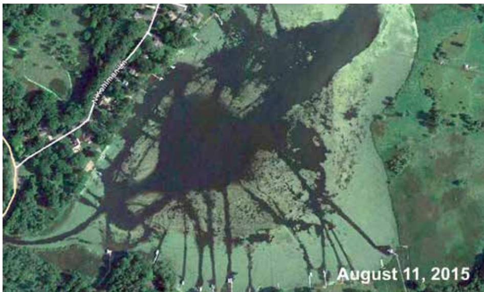
Figure 10. The aquatic plant harvester cut lanes to docks and also cleared an open water area in the center of the lake. Strips in the surfaced vegetation were evidence of the harvester's activity.
