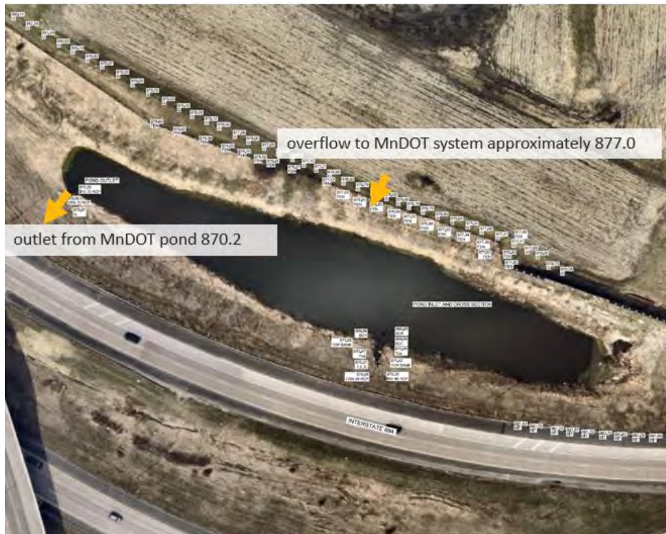
Figure 2-5 Watershed Overflow Location
