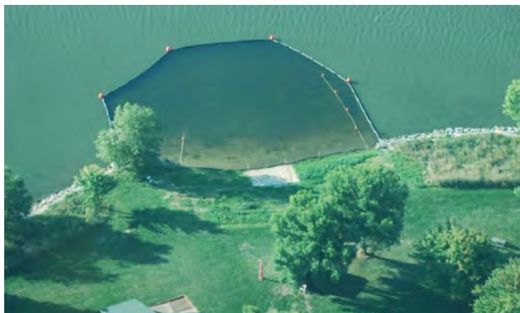
Figure 1: A Water Exclusion Treatment System installed at Brittingham Beach in Madison, Wisconsin [1]
