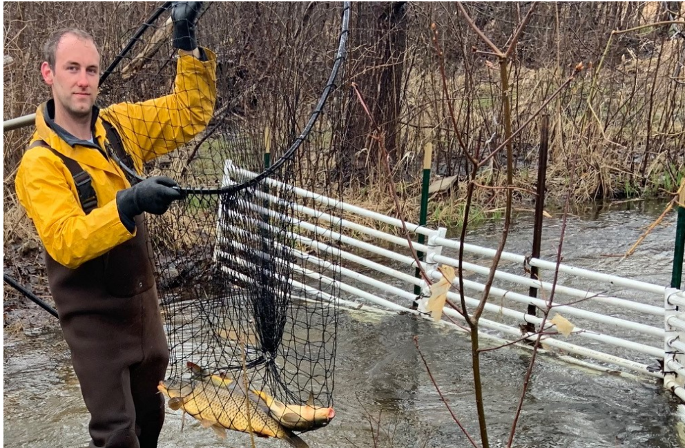
Figure 2: A simple PVC barrier was used to detect carp migration out of West Vadnais.
