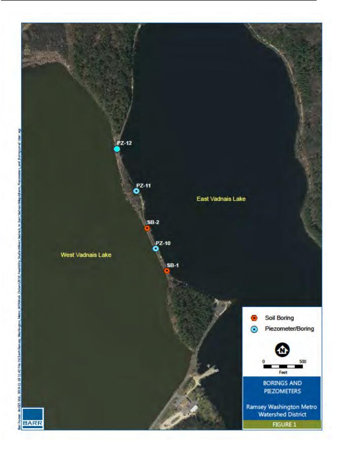
At three of the boring locations, piezometers were installed using hollow-stem-auger drilling methods. Each piezometers was installed to a depth of 8 feet, with a screened interval ranging from 3 to 8 feet below ground surface. The screened intervals intersect the water table, which varied from 3.1 feet to 3.6 feet below ground surface. Piezometer construction logs are presented in attachment A.
