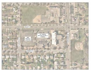
Figure 1: The St. Pascal Baylon Church project includes a tree trench and a rain garden that will remove phosphorus and sediment from stormwater that travels to Battle Creek.
